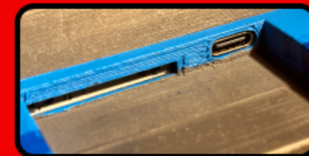
Back IO: USB-C port & SD card slot
